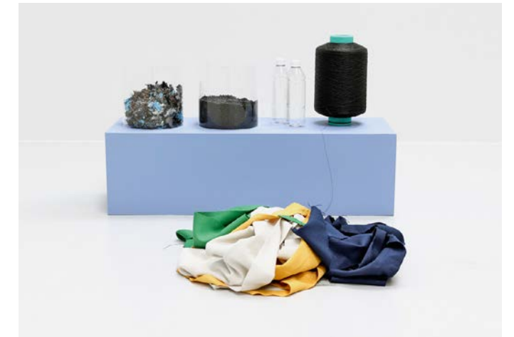
The textile waste is shredded, pelletized and mixed with recycled polyester from plastic bottles to create the yarn that is used for the Gabriel Loop fabric.
